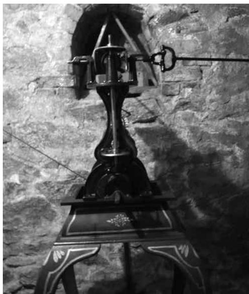
*The original Howard clock mechanism inside the tower of the Damon Memorial. The shaft on the right turns the clock hands on the east face of the tower. Hidden by the mechanism is the shaft driving the hands on the clock's north-facing dial.*
