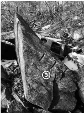
*Granite block at Dodd's quarry. Just above ③ are three shallow drill holes. Metal wedges and side pieces called feathers were inserted into these holes and then hammered to split the block.*
